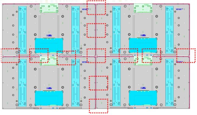
These bosses can be used to attach panels effectively.
