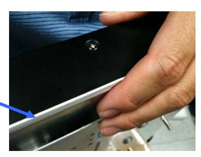
The frame is deeper than front bezel, so hands will not be injured by the slim edge of front bezel.
